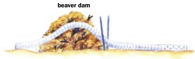
Figure 5-11. PVC Beaver Drain Pipe
