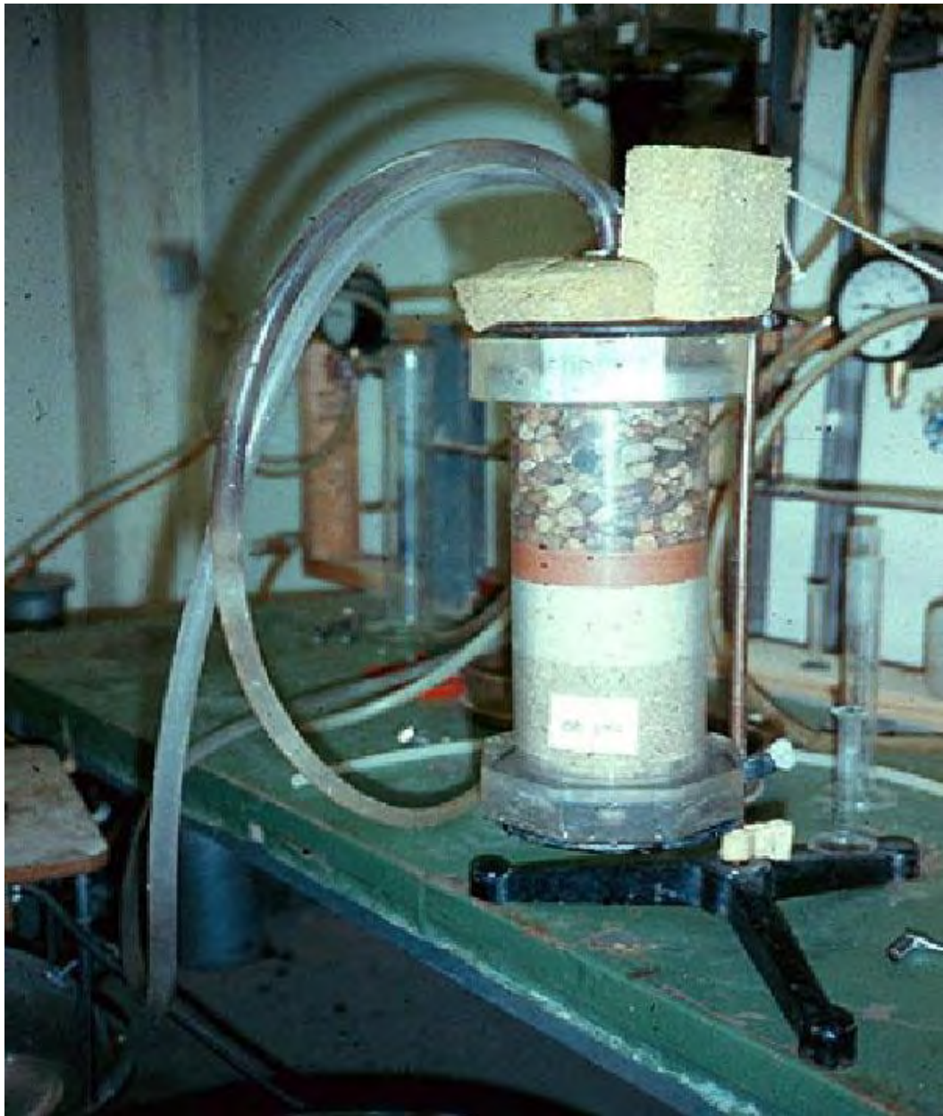
Figure F-4. No erosion filter test apparatus in Soil Conservation Service Laboratory in Lincoln, Nebraska. (Photo credit – James Talbot).
