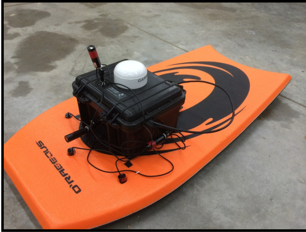
Figure 55: The bodyboard-mounted HDSS system.
