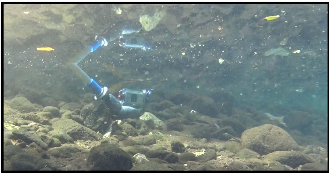
Figure 109: Underwater geo-referenced video camera used during the HDFS observations.
